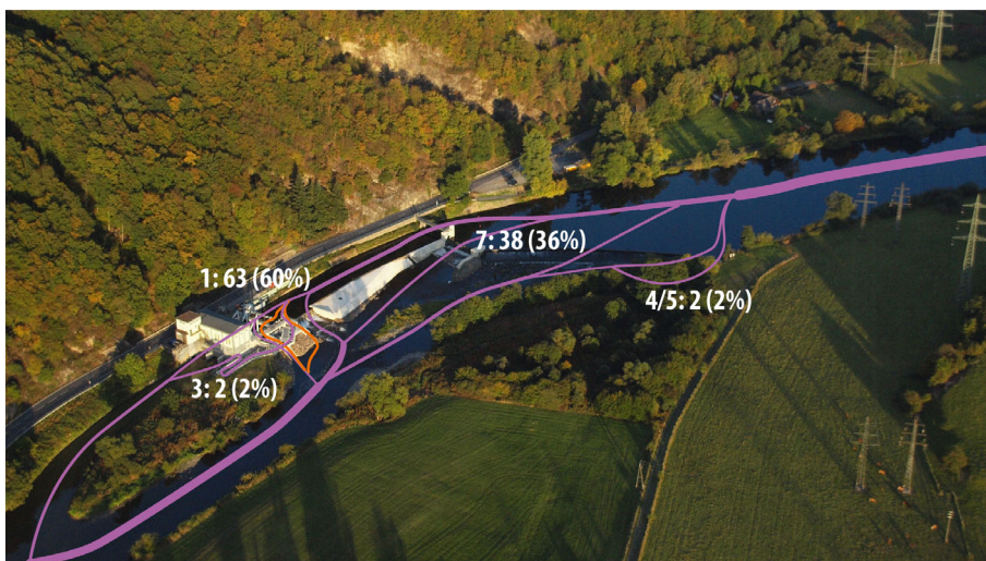
FIGURE 3 Number and proportion of smolts using the different migration routes past the power station. Route numbers refer to lower panel in Figure 2
