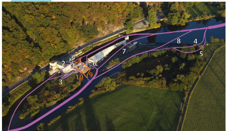
FIGURE 2 Upper panel: Migration routes available for downstream migrating fish at the weir: (1) via the side stream, (2) over the weir, (3) through the fence, or (4) through the fish trap, and then via (a) the vertical slot fishway, (b) natural fishway, or (c) ramp-like fishway or canoe pass. Lower panel: Migration routes available for downstream migrating fish at Unkelmühle power station: (1) via the surface bypass; custom-made openings in the racks that leads fish to a route outside the turbines via the flushing channel, (2) through turbines if they slip through the bar spacing of the racks, (3) through the vertical slot fishway constructed for upstream migrants, (4) through the nature-like fishway, (5) through the canoe pass, (6) via the ice gate, (7) over the spillway gate, (8) over the dam, (9) via the bottom bypass for eel, and (10) via side bypasses for eel (the two latter, indicated in orange, are only in operation during the eel run in the autumn). More detailed figures of the power station area can be found in Havn et al. (2018)
